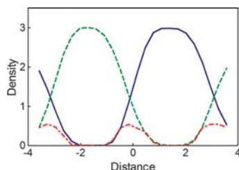
**Fig. 6** One-dimensional density profiles of the simulated PNC structure corresponding to a volume fraction of  $\phi_p = 0.2$  and a nanoparticle coverage PS<sub>1</sub>Au<sub>11</sub> in the direction perpendicular to the lamellae: PS (green), PVP (blue), Au (red).
