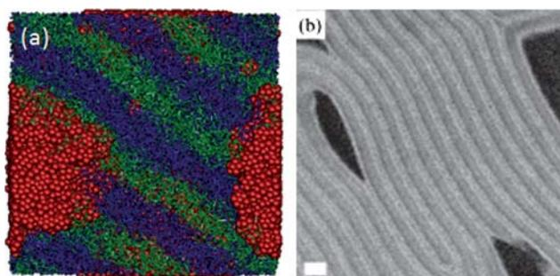
**Fig. 5** a: Snapshot of the simulated PNC structure corresponding to the PS<sub>4</sub>Au<sub>8</sub> nanoparticle coverage and volume fraction  $\phi_p = 0.20$ : PS-type beads (green), PVP-type beads (blue), Au nanoparticle beads (red). b: cross-sectional TEM image showing the macrophase separation of gold nanoparticles in symmetric PS-*b*-PVP block copolymers (reproduced from ref. 7 with permission of the American Chemical Society).
