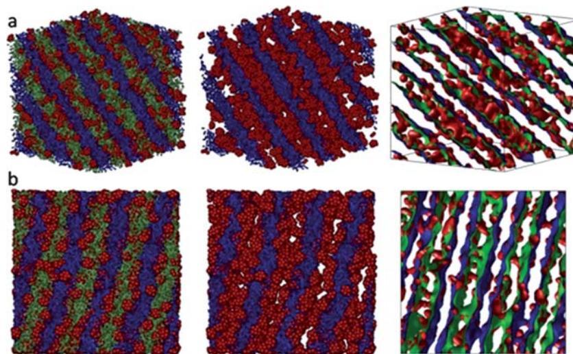
**Fig. 3** Left and middle columns: snapshots of the simulated PNC structures corresponding to a volume fraction of  $\phi_p = 0.1$  and to different nanoparticle coverage: a,  $\text{PS}_4\text{Au}_8$ ; b,  $\text{PS}_1\text{Au}_{11}$ . The PS domain was omitted from the snapshots in the central column for clarity. Right column: isosurface visualization of each component (PS, PVP and nanoparticles): PS-type beads (green), PVP-type beads (blue), Au nanoparticle beads (red).
