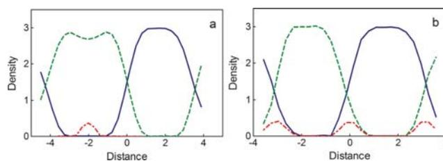
**Fig. 4** One-dimensional density profiles of the simulated PNCs with lamellar morphology and particles at  $\phi_p = 0.1$  in the direction perpendicular to the lamellae. Nanoparticle coverage architecture: a,  $\text{PS}_4\text{Au}_8$ ; b,  $\text{PS}_1\text{Au}_{11}$ . PS (green), PVP (blue), Au (red).
