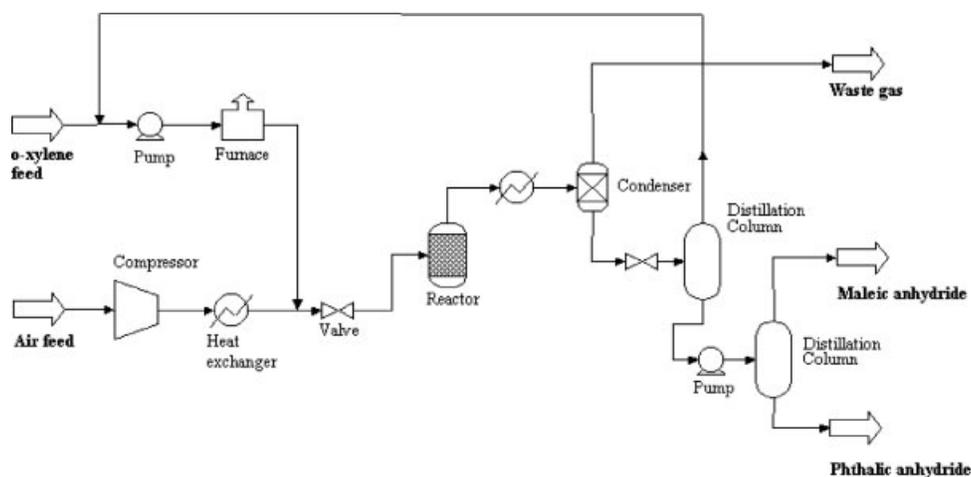
Figure 2. Production of phthalic anhydride from o-xylene.
