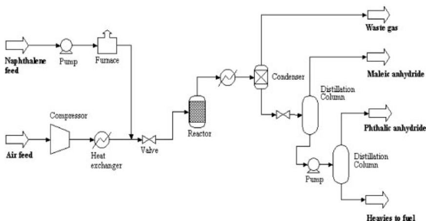
Figure 3. Production of phthalic anhydride from naphthalene.
