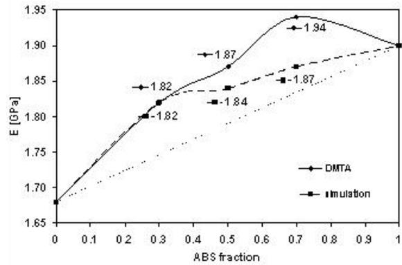
Fig. 3. Comparison between simulation and experimental values of storage modulus
