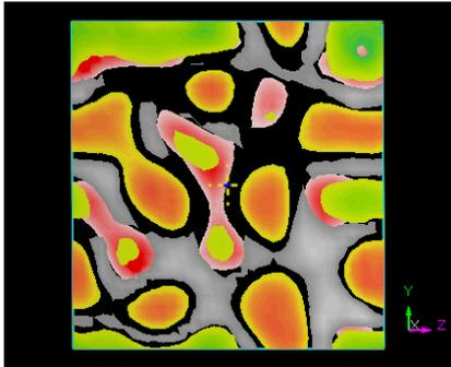
Fig. 1. Mesoscale section morphology of PC 15/ ABS 85 blends at 298K.
