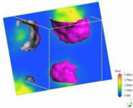
**Figure 3.** Isodensity surface and mapping of B-type beads (LDPE) onto a plane intercalated in the 3D cell for the systems PVC/LDPE system at 3% by weight of LDPE at 393 K and in the absence of shear.
