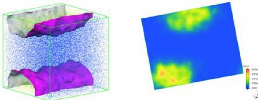
**Figure 4.** Isodensity surface and mapping of B-type beads (LDPE) onto a plane intercalated in the 3D cell for the systems PVC/LDPE system at 3% by weight of LDPE at 393 K under an applied shear rate of 100000 1/s.
