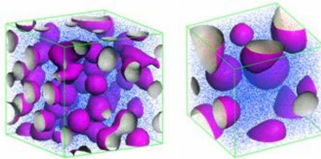
**Figure 1.** Isodensity surfaces for the PVC/LDPE system at 3% (left) and 10% (right) by weight of LDPE obtained from mesoscale simulations at 298 K and in the absence of shear.
