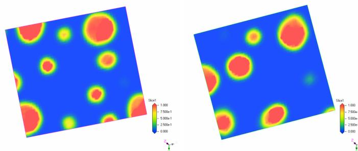
**Figure 2.** Mapping of B-type beads (LDPE) onto a plane intercalated in the 3D cell for the system PVC/LDPE system at 10% by weight of LDPE at 298 K and in the absence of shear. Right: after 5000 simulation steps; left: after 10000 simulation steps.
