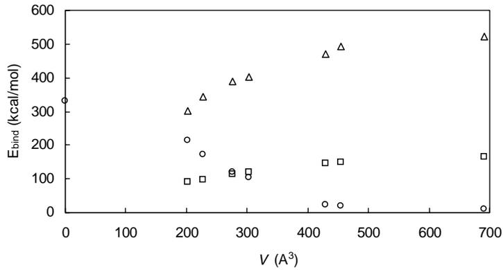
Fig. 6. Predicted  $E_{\text{bind}}$  vs. quat molecular volume  $V$ : (○)  $E_{\text{bind}}^{\text{MMT/nylon-6}}$ ; (□)  $E_{\text{bind}}^{\text{nylon-6/quat}}$ ; (△)  $E_{\text{bind}}^{\text{MMT/quat}}$ .
