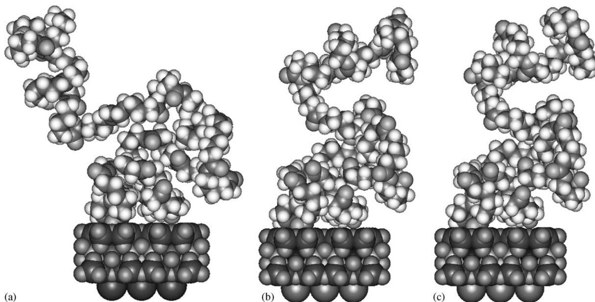
Fig. 2. Three frames extracted from a MD trajectory at  $T = 600$  K of a system made up by a pristine MMT platelet and a single nylon-6 polymer chain: (a) 0 ps; (b) 100 ps and (c) 250 ps.
