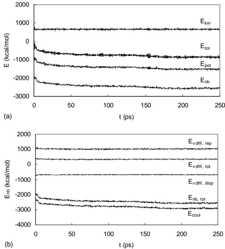
Fig. 3. Profiles of the energy components for the simulation shown in Fig. 2: (a) total energy and its components; (b) total nonbonded energy and its components.
