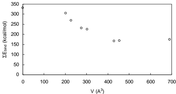
Fig. 7. Sum of  $E_{\text{bind}}^{\text{MMT/nylon-6}}$  and  $E_{\text{bind}}^{\text{nylon-6/quat}}$  vs. quat molecular volume  $V$ .
