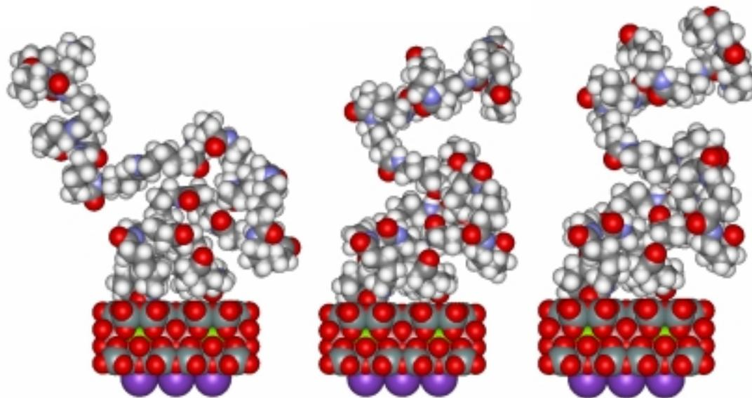
Fig.2. Three frames extracted from a MD trajectory at  $T = 600$  K of a system made up by a pristine MMT platelet and a single nylon-6 polymer chain. (left), 0 ps; (middle), 100 ps and (right), 250 ps.
