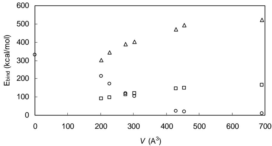
Fig. 6. Predicted  $E_{\text{bind}}$  vs. quat molecular volume  $V$ . (○),  $E_{\text{bind}}^{\text{MMT/nylon-6}}$ ; (□),  $E_{\text{bind}}^{\text{nylon-6/quat}}$ ; (Δ),  $E_{\text{bind}}^{\text{MMT/quat}}$ .
