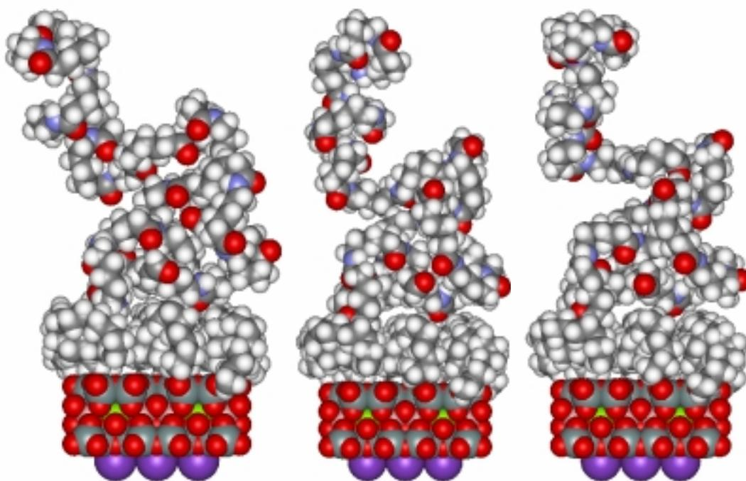
Fig. 4. Three frames extracted from a MD trajectory at  $T = 600$  K of a system of a system comprising the polymer and a MMT platelet exchanged with  $M_2(C_{18})_2$ . (left), 0 ps; (middle), 100 ps and (right), 250 ps.
