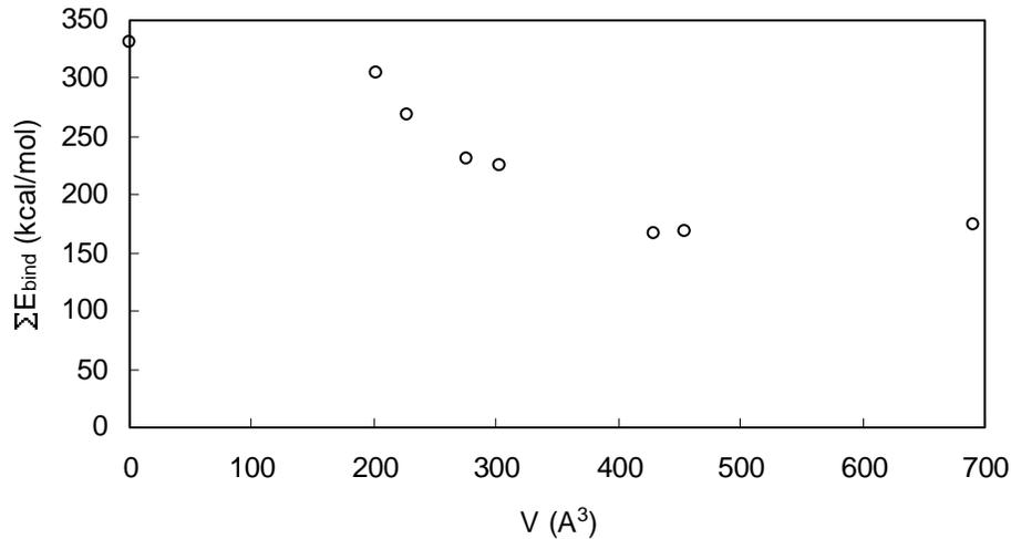
Fig. 7. Sum of  $E_{\text{bind}}^{\text{MMT/nylon-6}}$  and  $E_{\text{bind}}^{\text{nylon-6/quat}}$  vs. quat molecular volume  $V$ .
