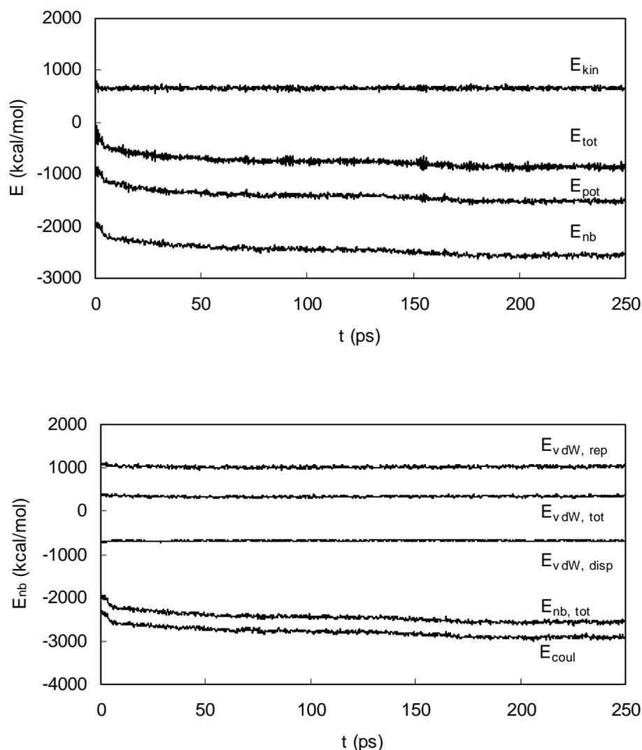
Fig. 3. Profiles of the energy components for the simulation shown in Figure 2. (top) total energy and its components; (bottom) total nonbonded energy and its components.
